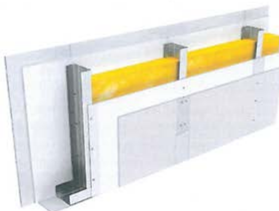
Figure 12 – Graphical representation of partition wall with two layers of NIDA plasterboard
