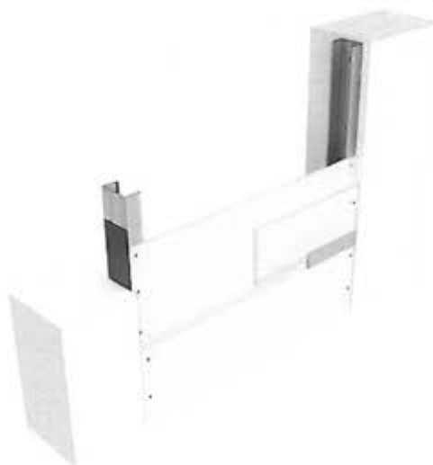
Figure 24 – Graphical representation of Shaft system with NIDA plasterboard
