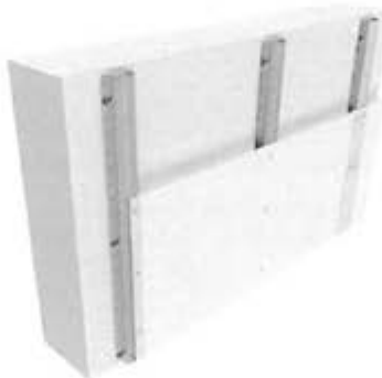
Figure 19 – Graphical representation of wall lining with NIDA plasterboard lining
