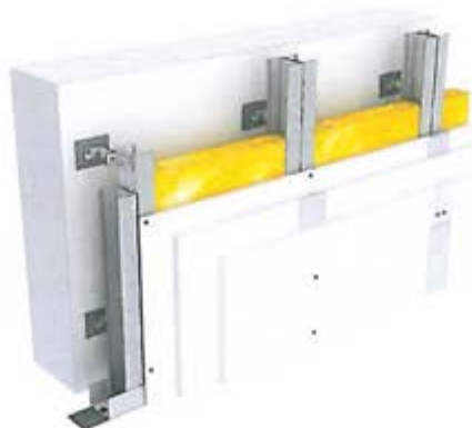
Figure 20 – Graphical representation of wall lining with NIDA plasterboard lining
