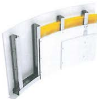
Figure 10 – Graphical representation of partition wall with two or three layers of NIDA plasterboard
