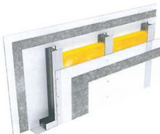
Figure 11 – Graphical representation of partition wall with two layers of NIDA plasterboard
