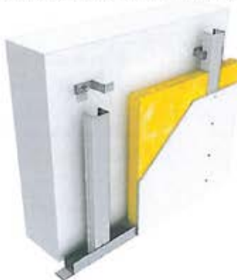
Figure 16 – Graphical representation of wall lining with NIDA plasterboard lining
