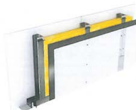
Figure 13 – Graphical representation of partition wall with one layer of NIDA RTG plasterboard
