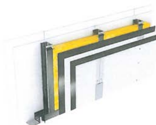
Figure 14 – Graphical representation of partition wall with two layers of NIDA RTG plasterboard
