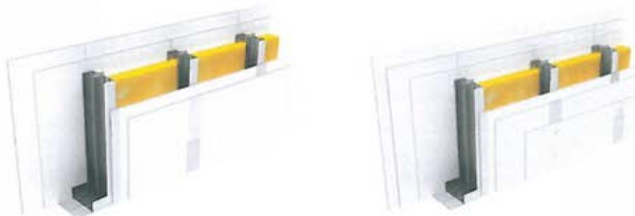
Figure 5 – Graphical representation of partition wall with two and three layers of NIDA plasterboard
