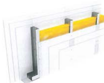
Figure 3 – Graphical representation of partition wall with three layers of NIDA plasterboard
