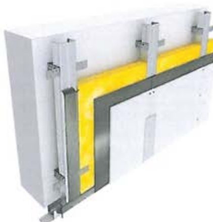
Figure 18 – Graphical representation of wall lining with NIDA RTG plasterboard lining
