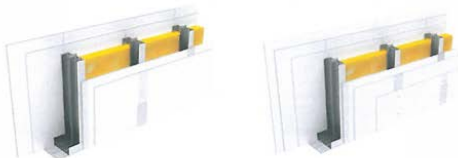
Figure 4 – Graphical representation of partition wall with two and three layers of NIDA plasterboard
