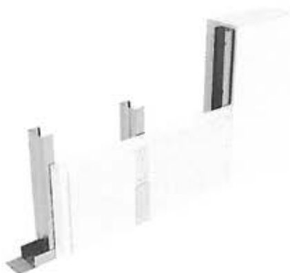
Figure 22 – Graphical representation of Shaft system with NIDA plasterboard
