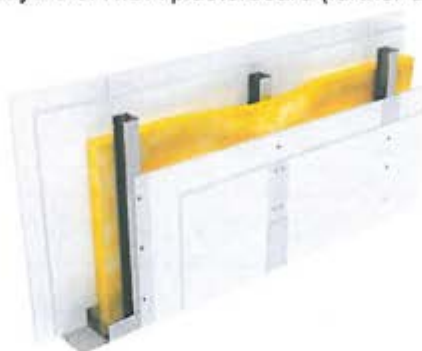
Figure 9 – Graphical representation of partition wall with two layers of NIDA plasterboard
