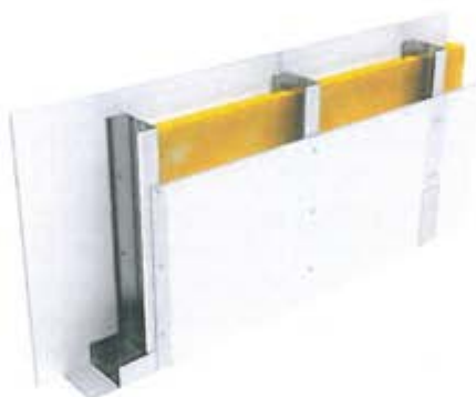
Figure 1 – Graphical representation of partition wall with one layer of NIDA plasterboard
