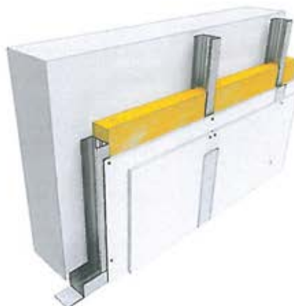
Figure 21 – Graphical representation of wall lining with NIDA plasterboard lining
