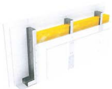
Figure 2 – Graphical representation of partition wall with two layers of NIDA plasterboard
