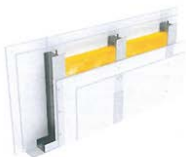
Figure 7 – Graphical representation of partition wall with two layers of NIDA plasterboard
