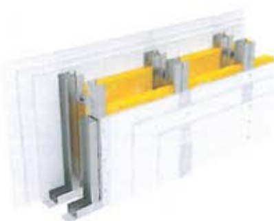
Figure 8 – Graphical representation of partition wall with three layers of NIDA plasterboard
