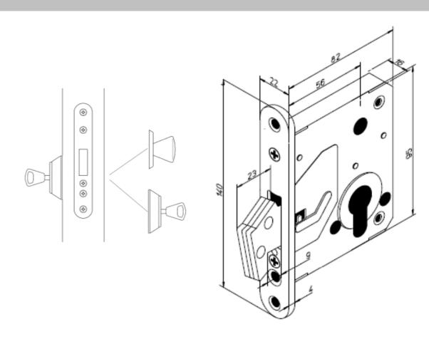
Security lock (comparable with security grade 4 according to EN 12209).
